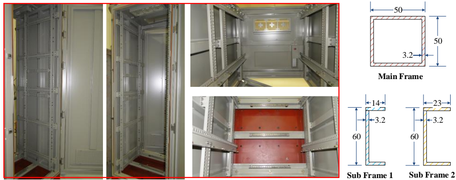
(c) Sections of frame elements [unit: mm]
