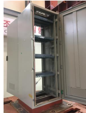
(b) Cabinet mount on shaking table test
