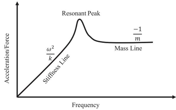
Fig. 5. Acceleration/force frequency response at resonance [24].
