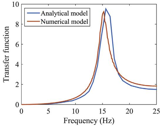
Fig. 8. Transfer function for analytical and numerical models.
