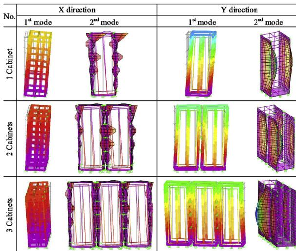
Fig. 10. Principal modes of vibration for three cases.
