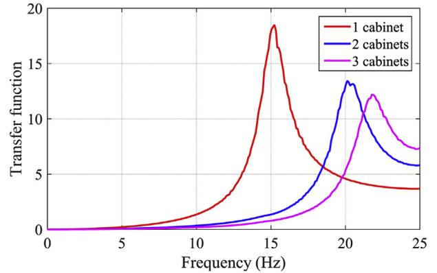
Fig. 14. Transfer function from the cabinet's response.
