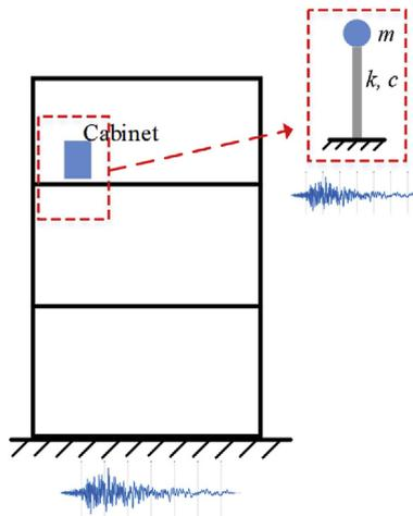
Fig. 4. Simplified model of the electrical cabinet.
